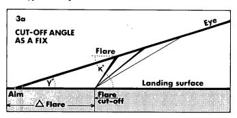
Calculation of this distance from the aim point to the flare cut-off point, ( $\Delta$  Flare), involves energy/geometry considerations, quickly determined in practice with experience, but complicated to derive by analysis.
