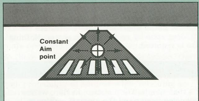
Points beyond the aim point will appear to move upward from the aim point, while points short of the aim point will appear to move downward. It is a point in this 'six o'clock' sector of the pilots' view which has proven useful.
