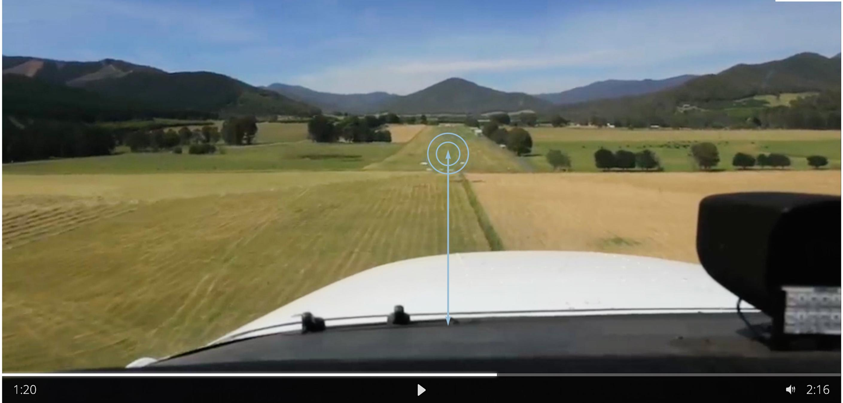
**Short final: Maintaining work cycle:** Aim point relationship – Centreline – Flight path angle – Airspeed.
