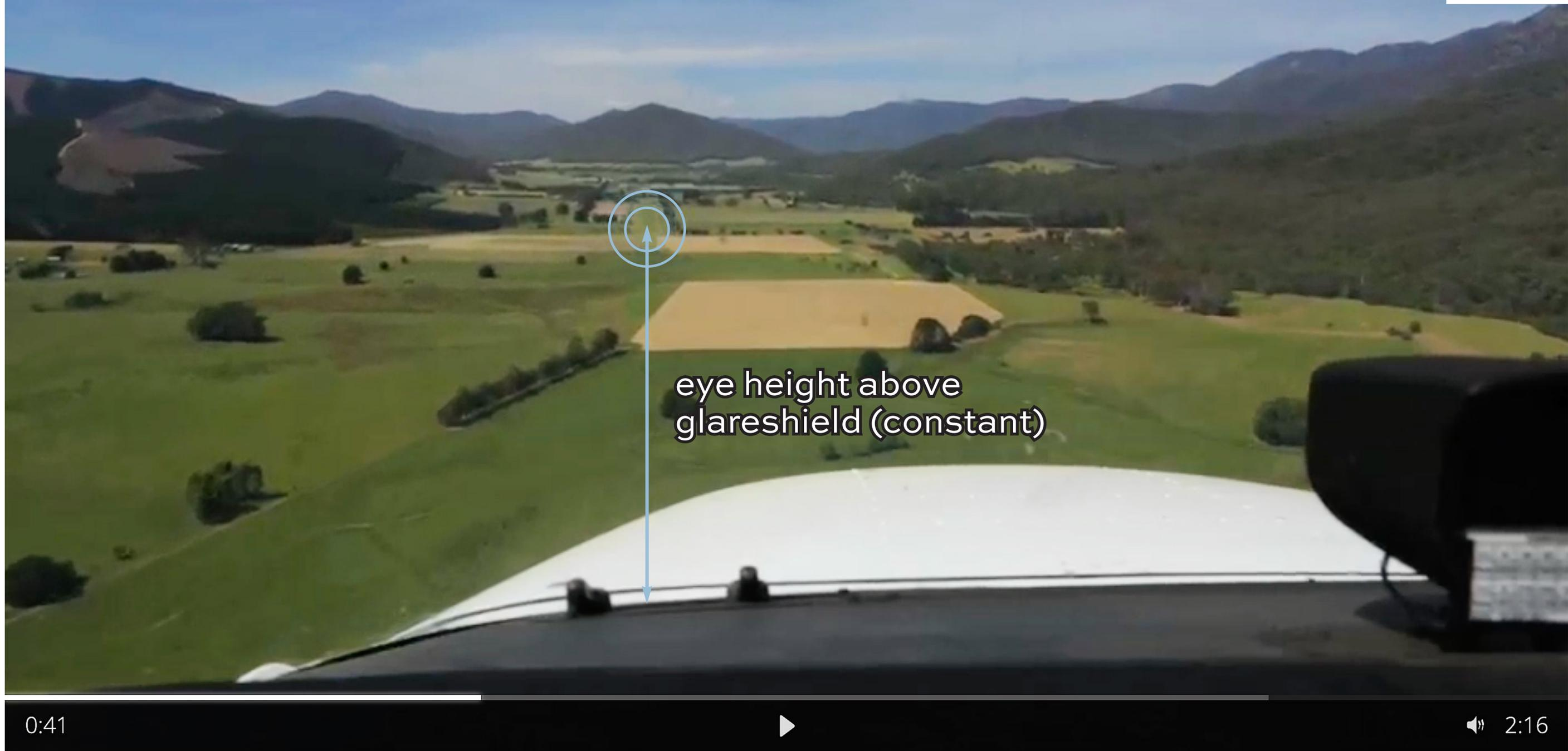
Joining 2nm final around 600ft above runway threshold on airstrip centreline, configured for approach.
