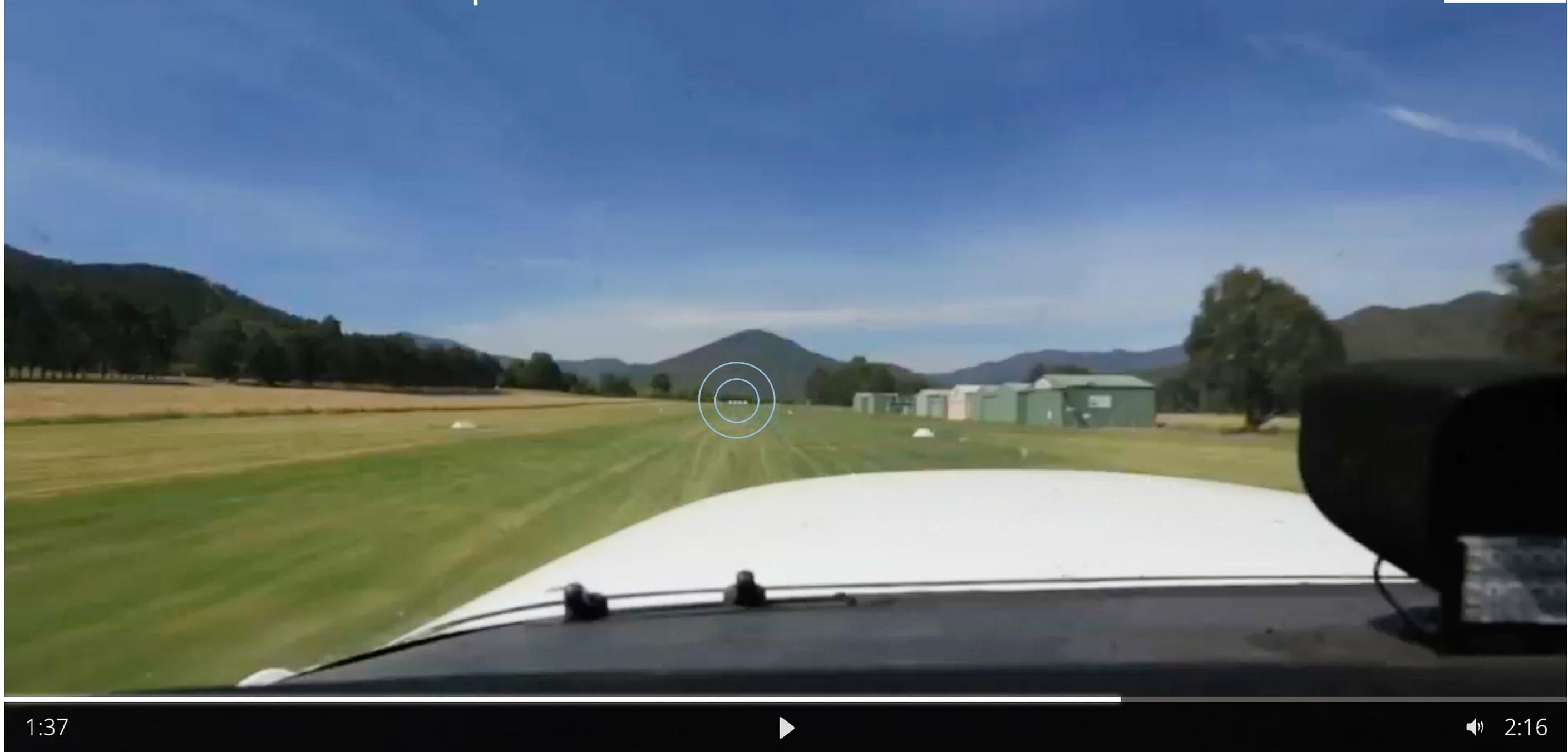
**Touchdown:** If the approach was well stabilised, the approach IAS was flown accurately, and the 4-second flare completed as described, then touchdown should occur between 4-6 seconds after the flare commencement, with the touchdown located very close to the original aim point 1. Continue to use judicious inputs on all flight controls through the continuing rollout, until runway turn-off. Test brakes gently, applying as necessary to make the desired turn-off point at a safe speed.
